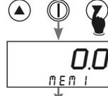
When desired memory location is displayed, take the pressure reading. The peak reading will be captured.
