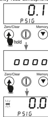
Continue to press the Zero/Clear button until *0000* is displayed then release the button. The gauge is now zeroed.
