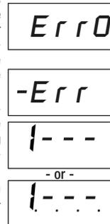
If excessive vacuum is applied to a pressure-only gauge, the display will indicate *-Err* until the vacuum is released. Applying vacuum to a pressure-only gauge can damage the pressure sensor.
